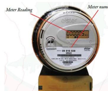
The typical electrical meter above shows where to read the amount of electricity consumed.
